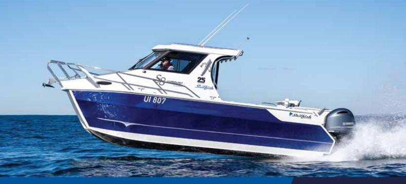
Hull L.O.A – 7.9m / L.O.A on trailer – 8.5m / Beam – 2.45m Height on trailer – 3.50m / Fuel – 2 x 190L tanks / Built-in foam buoyancy
