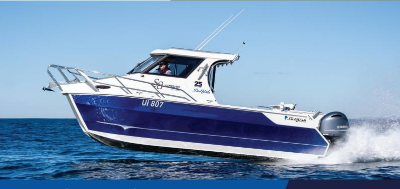
Hull L.O.A - 7.9m / L.O.A on trailer - 8.5m / Beam - 2.45m Height on trailer - 3.50m / Fuel - 2 x 190L tanks / Built-in foam buoyancy
