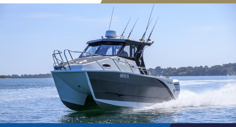
Hull L.O.A - 7.3m / L.O.A on trailer - 8.1m / Beam - 2.45m / Height on trailer - 3.45m Fuel - 2 x 190L tanks / Built in foam buoyancy
