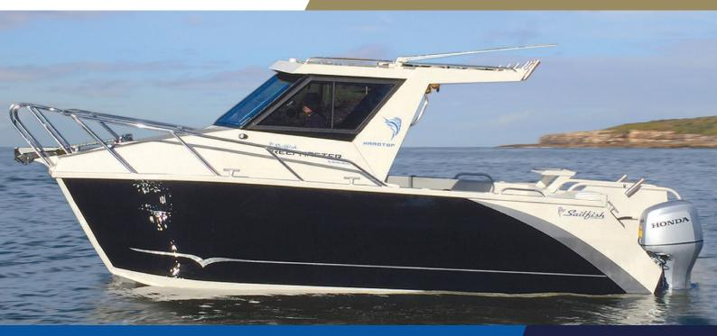
Hull L.O.A - 7.3m / L.O.A on trailer - 8.1m / Beam - 2.45m Height on trailer - 3.45m / Fuel - 2 x 190L fuel tanks / Built-in foam buoyancy
