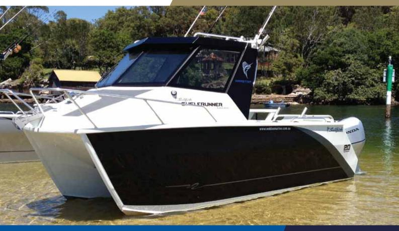
Hull L.O.A - 6.9m / L.O.A on trailer - 7.5m / Beam - 2.45m / Height on trailer - 3.40m Fuel - 2 x 170L fuel tanks 5mm hull, 3mm sides and cabin / Built-in foam buoyancy
