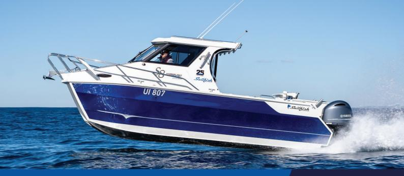
Hull L.O.A – 7.9m / L.O.A on trailer – 8.5m / Beam – 2.45m Height on trailer – 3.50m / Fuel – 2 x 190L tanks / Built-in foam buoyancy
