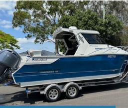
SPECIFICATIONS Hull L.O.A - 7.3m L.O.A on trailer - 8.1m Beam - 2.45m Height on trailer - 3.45m Fuel - 2 x 190L tanks Hull Thickness - 5mm / Sides Thickness - 3mm Pax Capacity - 7 Built-in Foam Buoyancy
