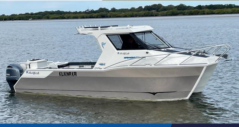
Hull L.O.A - 8.20m / L.O.A on trailer - 9.30m / Beam - 2.45m Height on trailer - 3.45m / Fuel - 2 x 190L tanks / Built-in foam buoyancy
