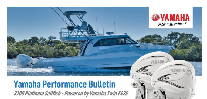
Performance SummaryTest Date: 13 Jul 2022Max. Ave Speed71.3 Km/h or 38.4307 KnotsBest Cruising Km/L0.41 Km/L @ 3500 RPMRange based on 95% Fuel Capacity at Best Km/L470 Kilometres
