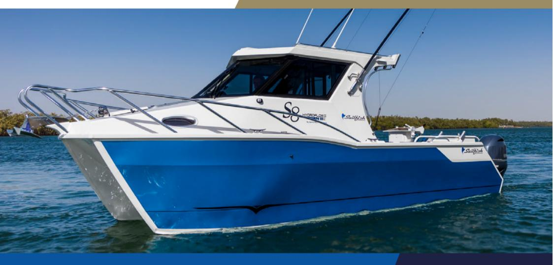
Hull L.O.A - 7.9m / L.O.A on trailer - 9.0m / Beam - 2.45m Height on trailer - 3.50m / Fuel - 2 x 190L tanks / Built-in foam buoyancy
