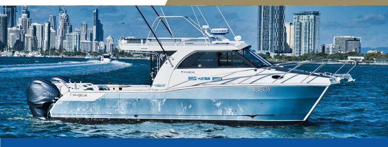
Hull LOA - 10.6m / Beam - 3.00m (Optional 3.50m Beam) / Fuel Capacity - 2 x 300L Tanks (3.50m beam - 2 x 500L Tanks) / Water Tank - 200L / Draught - 600mm (approx.) / Built In Foam Buoyancy
