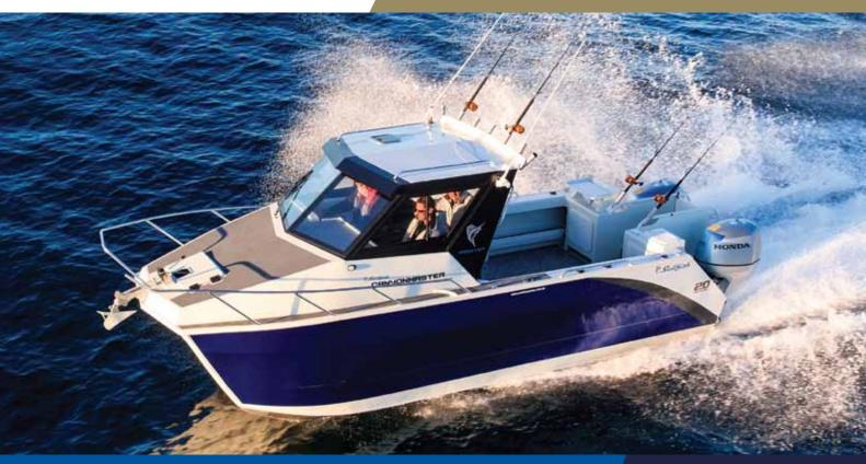
Hull L.O.A - 7.9m / L.O.A on trailer - 8.5m / Beam - 2.45m Height on trailer - 3.45m / Fuel - 2 x 190L tanks / Built-in foam buoyancy
