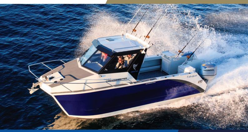
Hull L.O.A - 7.9m / L.O.A on trailer - 8.5m / Beam - 2.45m Height on trailer - 3.45m / Fuel - 2 x 190L tanks / Built-in foam buoyancy
