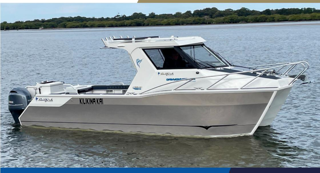
Hull L.O.A - 8.20m / L.O.A on trailer - 9.30m / Beam - 2.45m Height on trailer - 3.45m / Fuel - 2 x 190L tanks / Built-in foam buoyancy
