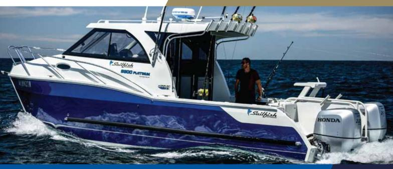
Hull L.O.A - 8.8m / L.O.A on trailer - 9.7m / Beam - 2.8m / Height on trailer - 3.7m Fuel - 2 x 240L tanks / Holding tank - 25L / Water tank - 110L / Built-in foam buoyancy / Passengers - 9
