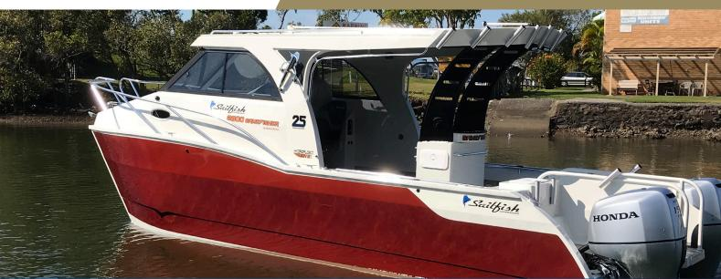
Hull L.O.A - 8.8m / L.O.A on trailer - 9.7m / Beam - 2.5m / Optional beam - 2.8m / Height on trailer - 3.67m Fuel - 2 x 240L tanks /Water tank - 60L / Built-in foam buoyancy / Draft approx. - 600mm / Passengers - 9
