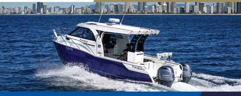
Hull L.O.A - 8.8m / L.O.A on trailer - 9.7m / Beam - 2.5m / Optional beam - 2.8m / Height on trailer - 3.67m Fuel - 2 x 240L tanks / Water tank - 60L / Built-in foam buoyancy / Draft approx. - 600mm / Passengers - 9
