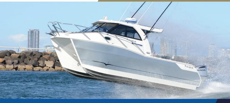
Hull L.O.A - 9.4m / L.O.A on trailer - 10m / Beam - 2.8m / Height on trailer - 3.7m / Fuel - 2 x 300L tanks Water tank - 200L Holding tank - 48L / Passengers - 9 / Draft approx. - 600mm / Built-in foam buoyancy
